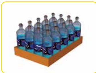
Hot melt glue is applied and the tray's (major) flaps are folded up, compressed and sealed.
