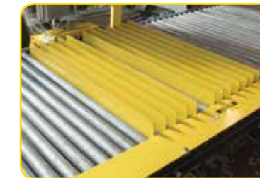
Pallet Lift Mechanism in Wrap Zone Provides Lower Wrap Heights
