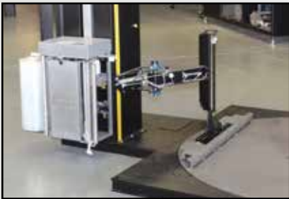
Clamp, Cut and Wipe Down System
