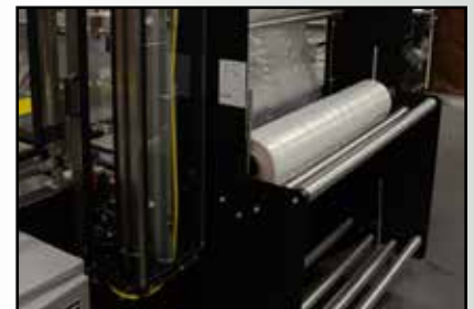
Side Mounted Dual Film Cradles for Easy Film Loading
