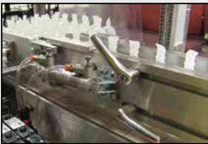
Fast Tool-Less Changeovers with Scales and Adjustable Handles
