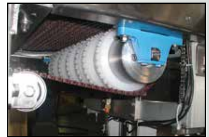
Motorized Pulleys Replace Greasy Chains
